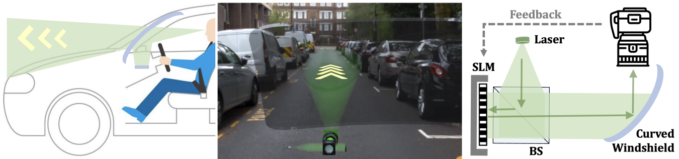
Figure 1: Conceptual illustration of a holographic HUD that applies to windshield AR navigation scenarios and supports multi-plane display experience, leveraging an off-the-shelf free-form geometry optical combiner, which can be compensated by a learning-empowered, calibrated hologram generation algorithm to deliver virtual 3D scenes without distortion.
